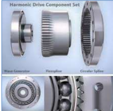
Figure 2. Description of harmonic gear drive
